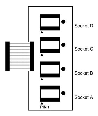
NOTE: Align PIN 1 of 28 pin devices with the arrow indicated.
