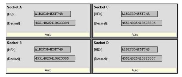
**Manual Serial Numbers** - Serial numbers can be entered manually for each device by unselecting the "Auto" check box and editing the HEX or Decimal field beside each socket identifier. The "Last HEX" and "Last Decimal" fields will reflect the last value used to serialize a device.
