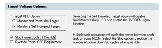
Modify this setting for In-Circuit Programming to select whether QuickWriter supplies the power for the target circuit or whether the Target circuit will supply its own power. (see: ICP with Self Powered Targets 21)
