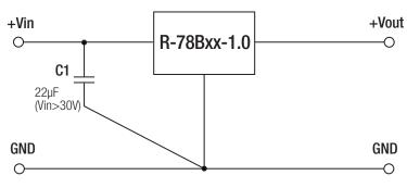
To protect the converter during power-up, use  $C1=22\mu F$  if Vin>30V
