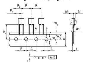
Figure 2 — Lead Spacing 7.5 mm
