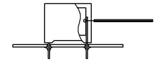
Temperature monitored inside the capacitor.
