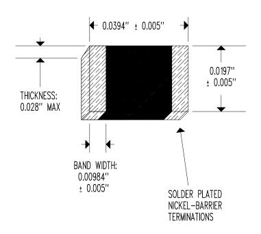
RESISTANCE @  $+25^{\circ}\text{C} = 10,000 \ \Omega \pm 5\%$ RESISTANCE/TEMPERATURE CURVE = "J" BETA " $\beta$ " (+25 TO  $+85^{\circ}\text{C}$ ) = 3,976 K NOMINAL TEMPERATURE COEFFICIENT @  $+25^{\circ}\text{C} = -4.4\%$ /C NOMINAL OPERATING TEMPERATURE RANGE = -40 TO  $+125^{\circ}\text{C}$
