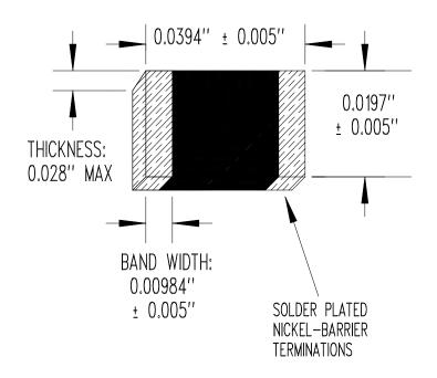
RESISTANCE @  $+25^{\circ}\text{C} = 10,000 \ \Omega \pm 1\%$  ACCURACY @  $+25^{\circ}\text{C} = \pm 0.23^{\circ}\text{C}$  RESISTANCE/TEMPERATURE CURVE = "J" BETA " $\beta$ " (0 TO  $+50^{\circ}\text{C}$ ) = 3,900°K NOMINAL TEMPERATURE COEFFICIENT @  $+25^{\circ}\text{C} = -4.4\%$ /°C NOMINAL OPERATING TEMPERATURE RANGE = -40 TO  $+125^{\circ}\text{C}$
