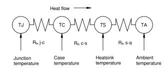
Thermal resistance:  $R_{th}$  j-c = junction to case
