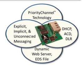
EtherNet/IP support includes Dynamic Host Configuration Protocol (DHCP) and Address Conflict Detection (ACD). Together, these two
