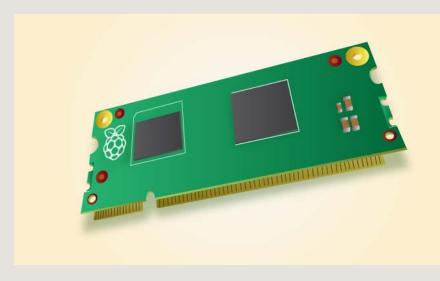
The Compute Module is a Raspberry Pi in a more flexible form factor, intended for industrial application.
