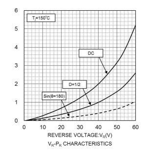
REVERSE POWER DISSIPATION:P<sub>R</sub>(mW)
