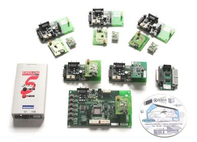
Zensys' Z-Wave<sup>™</sup> Developer's Kit v4.x enables developers and Original Equipment Manufacturers (OEMs) to design, and develop products that network wirelessly using the RF based Z-Wave Technology.
