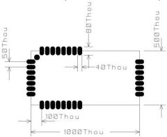
A PCB with two or more layers and with a solid ground plane in one of the inner- or bottom layer(s) is recommended. All GND-pins of the module shall be connected to this ground plane with vias with shortest possible routing, one via per GND-pin.
