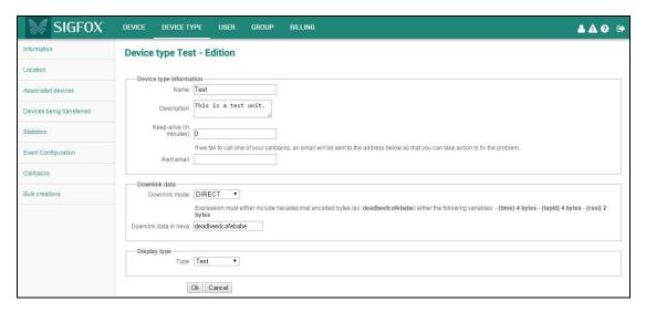
Step 5. Edit the Downlink data in hexadecimal entry as the payload of reply.
