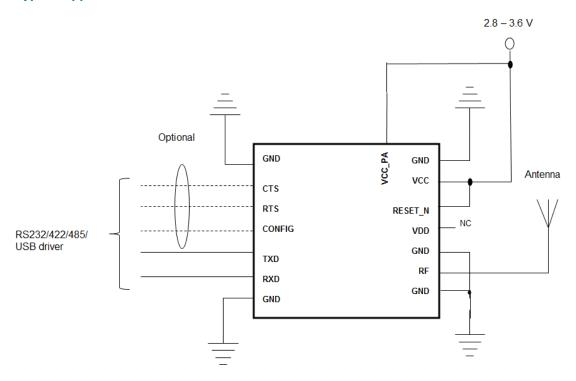
Note that the VCC\_PA pin supply the internal power amplifier only while the rest of the internal block runs on VCC. They can be connected together or separated using individual supply. For the RC1701 variant the VCC\_PA pin can be left open.
