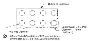
For .006" Thick Solder Paste Stencil, Aperture Opening Should be Equal to the PCB Pad Diameter.
