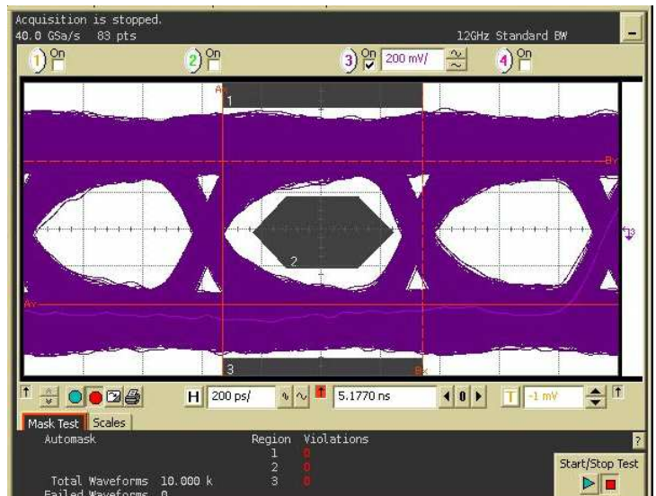
Figure 3 - Typical HDMI 1.3 Eye Pattern (1080p) with RClamp0524PA
