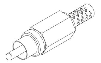
SPECIFICATIONS: CONTACT RESISTANCE: 30m OHMS MAX INSULATION RESISTANCE: 100M OHMS MIN: 500V DC VOLTAGE WITHSTAND: 500V AC R.M.S. FOR 1 MINUTE LIFE: 5,000 CYCLES OPERATING TEMP: -20° ~ +85°C
