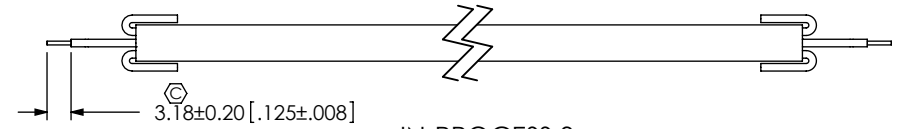
IN-PROCESS 3 STRIP INDIVIDUAL WIRES AND DIP IN TIN
