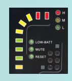
Extech's Refrigerant Leak Detector is easy to use and is ideal for detecting leakages from air-conditioning units and cooling systems that use all standard refrigerants. The multicolored LED light bar indicates the level of leaking refrigerant detected by the RD300. The built-in, bright LED convenience light located at the sensor tip illuminates dimly lit inspection areas.
