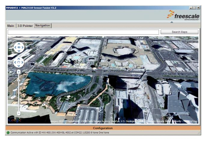
The Navigation screen uses all three angles output from the sensor daughter board to control the Google Maps display. The roll angle controls the display in the left and right direction. The pitch angle controls the display in forward and backward direction. The compass/yaw angle controls the rotation of the map display.
