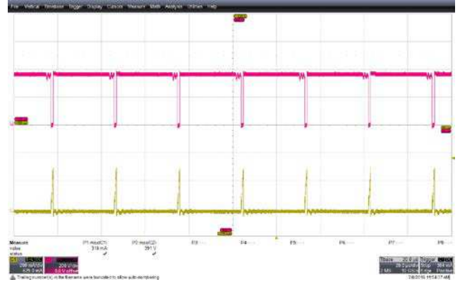
Figure 14 – Drain Voltage and Current Waveforms. 265 VAC, 120 mA Output. V_{DS(Max)} : 391 V. Upper: V_{DRAIN} , 200 V, 20 \mu s / div. Lower: I_{DRAIN} , 200 mA / div.
