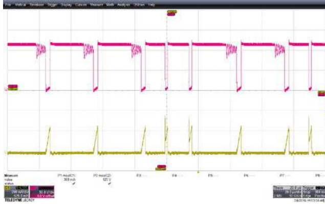
Figure 13 – Drain Voltage and Current Waveforms. 85 VAC, 120 mA Output. Upper: V_{DRAIN} , 50 V, 20 \mu s / div. Lower: I_{DRAIN} , 200 mA / div.
