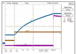
FIGURE 3-1: RE46C317 Horn Turn-On Delay.
