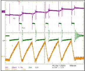
FIGURE 3-2: RE46C317/18 Switching Waveforms.
