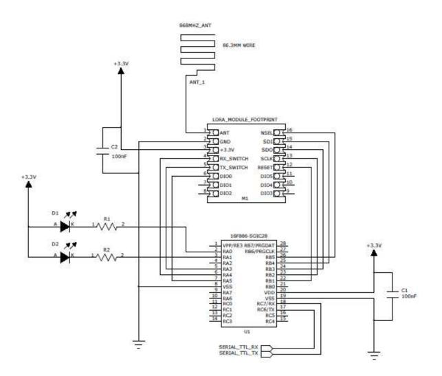
The above schematic shows an easy interface to a PIC Microcontroller
