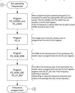
A total of four registers must be programmed to set the device operating frequency. This will take 5.2 us for each path at maximum clock speed.
