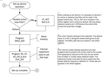
Three registers need to be written, taking 3.9us at the maximum clock speed. If the device is used with an active filter in simplex operation it will not be necessary to program CFG1 reducing the programming time to 2.6us.
