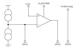
The charge pump output voltage compliance range is typically +0.7V to +1.5V. For applications using a passive loop filter VCO coarse tuning must be performed regularly enough to ensure that the VCO tuning voltage falls within this compliance range at all temperatures. The active loop filter maintains the charge pump output voltage in the center of the compliance range, and the op-amp provides a wider VCO tuning voltage range, typical OV to +2.4V.
