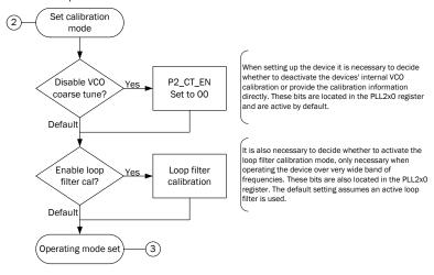
Two registers need to be written taking 2.6us at maximum clock speed if the course tuning is deactivated or the loop filter calibration activated. Since it is necessary to program these registers when setting the operating frequency (see next section) this operation usually carries no overhead.
