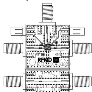
Broadband Application Circuit (500MHz to 4000MHz) - all capacitors are 100pF. Operation outside this band requires re-optimization of the capacitors.
