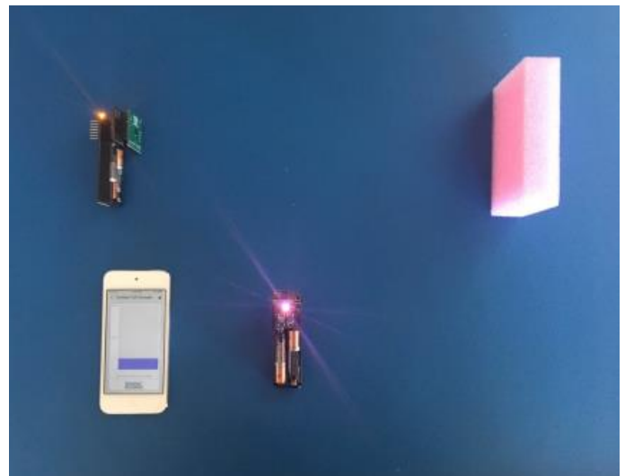
Figure 28 - ToF measurement with SimbleeForMobile and Paired Node - Farther Distance
