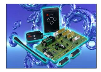
The RFEVAL2 / RFEVAL3 are hardware development platforms designed to assist the engineer design a remote telemetry application. Each project uses the advanced RF600E and RF600D Keeloq protocol and a variety of radio modules. Our aim with this Evaluation kit is to assist the engineer in designing a remote telemetry application with optimum Range.
