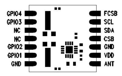
Figure 2. Pin Diagram
