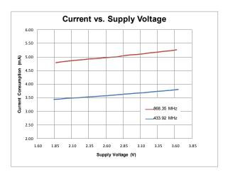
Figure 3. Current vs. Voltage,  $F_{RF} = 433.92 /$ 868.35 MHz, OOK, SR = 1 ksps
