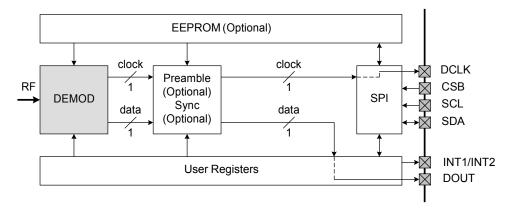
Figure 20. Data Path of Direct Mode
