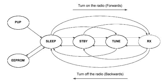
Figure 17. Device Operating State Machine
