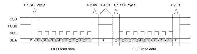
Figure 15. SPI Read FIFO Timing
