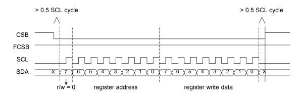
Figure 14. SPI Write Register Timing
