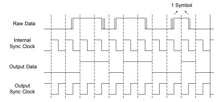
Figure 21. Demodulated Data and Sync Clock Timing Characteristics
