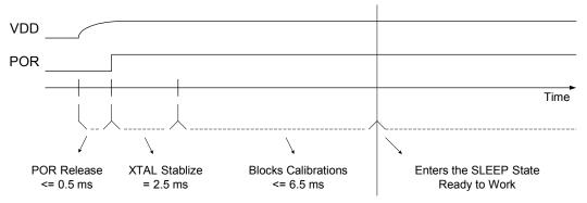
Figure 16. Power-Up Sequence Timing
