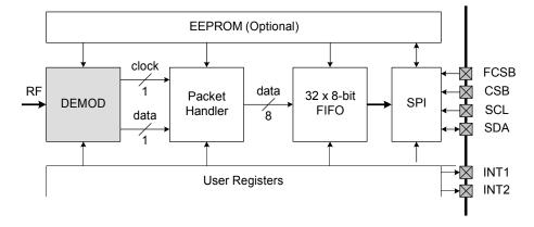
Figure 23. Data Path of Packet Mode
