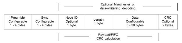
Figure 25. Variable Length Packet Structure
