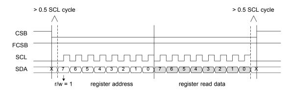
Figure 13. SPI Read Register Timing
