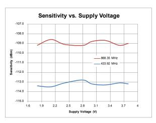
Figure 5. Sensitivity vs. Supply Voltage, SR = 1 ksps, OOK, BER = 0.1%
