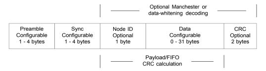
Figure 24. Fixed Length Packet Structure
