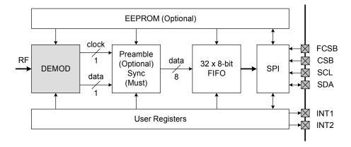
Figure 22. Data Path of Buffer Mode
