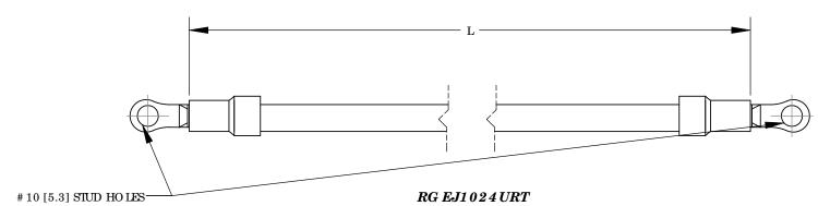
FAC TO RY C RIMPED # 10 AWG/6mm SQ . JUMPER WIRE ASSEMBLY (Q TY. 1) INC LUDES: PV10-10RX (Q TY. 2) # 10 AWG/6mm SQ . WIRE - G REEN/YELLO W INSULATIO N
