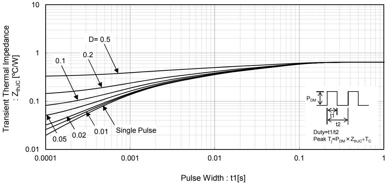
Fig.17 IGBT Transient Thermal Impedance
