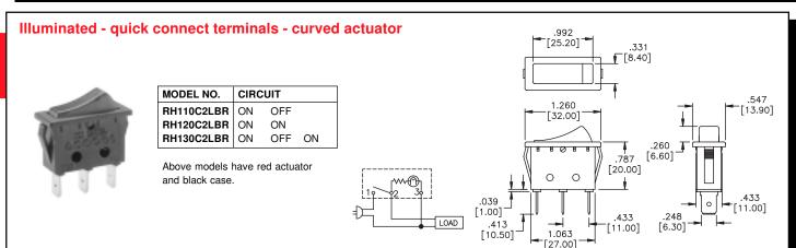
**Additional ordering information:** Commonly ordered models are shown above with complete model numbers and specifications. Below is an order format that enables you to 'build your own switch' and specify the correct switch model number by simply selecting from all available options shown and filling in the boxes.
