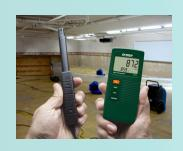
Compact handheld Hygro-Thermometer with large dual LCD displays Temperature and Humidity or Dew Point simultaneously. Dew Point measurement can indicate if conditions are suitable for painting. Ideal for many industrial applications or home use.
