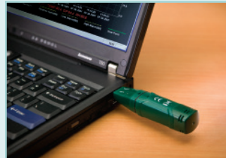
USB connector easily plugs into a computer for data analysis of Temperature and Humidity
