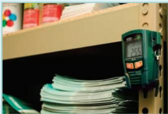
Monitors Humidity and Temperature levels in warehouse, storage rooms, freezers, shipping vans, and offices
