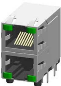
P/N RJSAE-5385-02 SHOWN STACKED 2x1, 8 POSITION, WITH SHIELD AND LEDS
