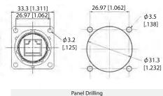
■ Jam nut receptacle • Hexagonal Nut mounting: Shell type 7
