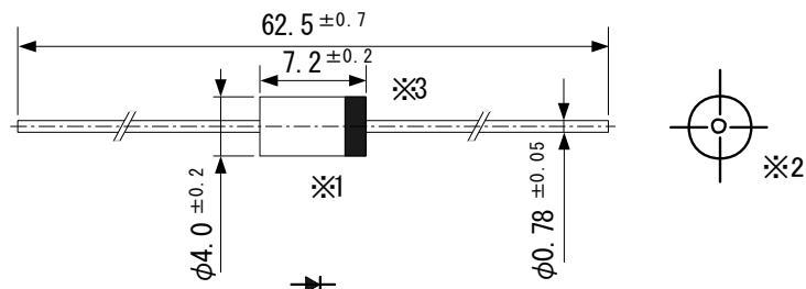
\*1 The allowance position of Body against the center of whole lead wire is 0.5mm(max.)
