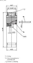
connector 3-, 4-, and 5-pole with threaded joint, assembling with screw terminals.
