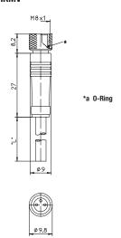
Actuator/sensor cordset, single-ended, M8, 3-, 4-, and 8-poles, female 90° connector with self-locking threaded joint and molded cable.
