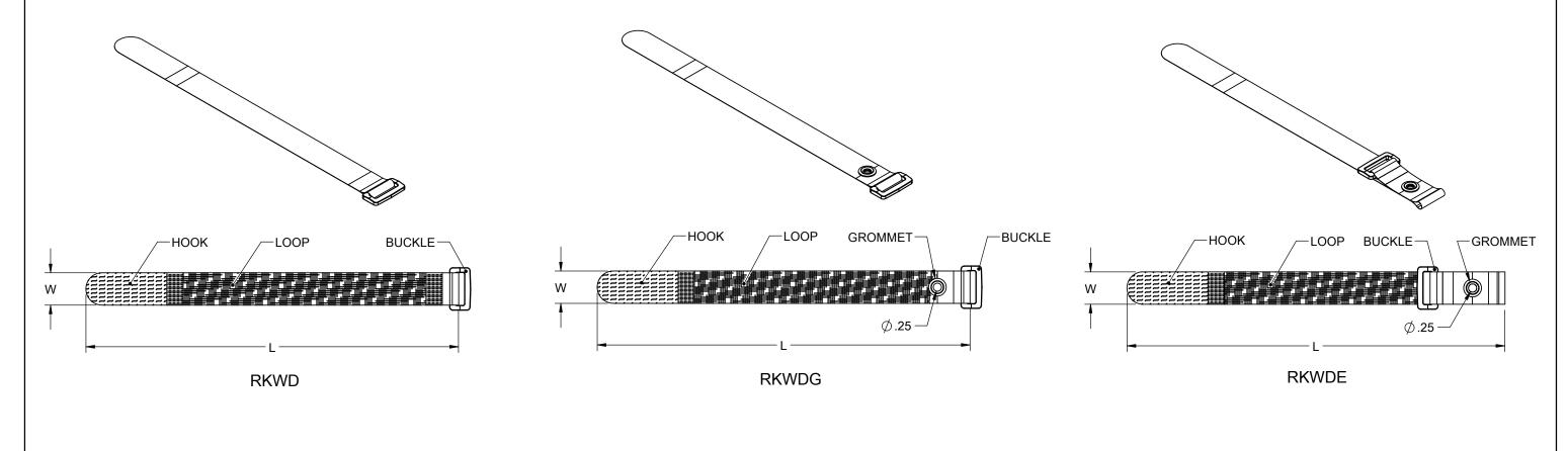
NOTES: 1. MATERIAL: HOOK & LOOP: NYLON WOVEN GROMMET: BRASS WITH BLACK OXIDE FINISH BUCKLE: NYLON, COLOR: BLACK
