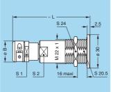
$\label{eq:Note:Chrome-plated brass outer shell, PTFE insulator, solder female contact, cable clamping, soldered external shield (part number ending with "S").}$
