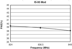
RMPA0967 Cellular 3x3mm<sup>2</sup> PAM Vcc=3.4 V, Vref=2.85V, Vmode=0V, Pout=28 dBm,
