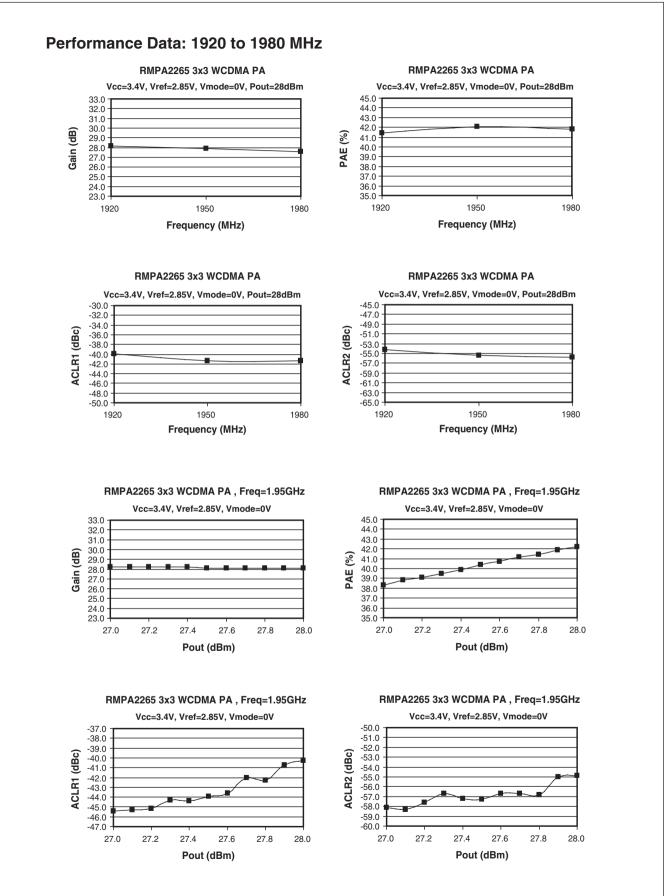
RMPA2265 Dual Band WCDMA Power Edge<sup>™</sup> Power Amplifier Module 1850 to 1910 MHz and 1920 to 1980 MHz
