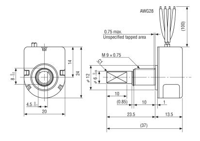
Unless otherwise specified, tolerance:  $\pm$  0.4 (Unit: mm)
