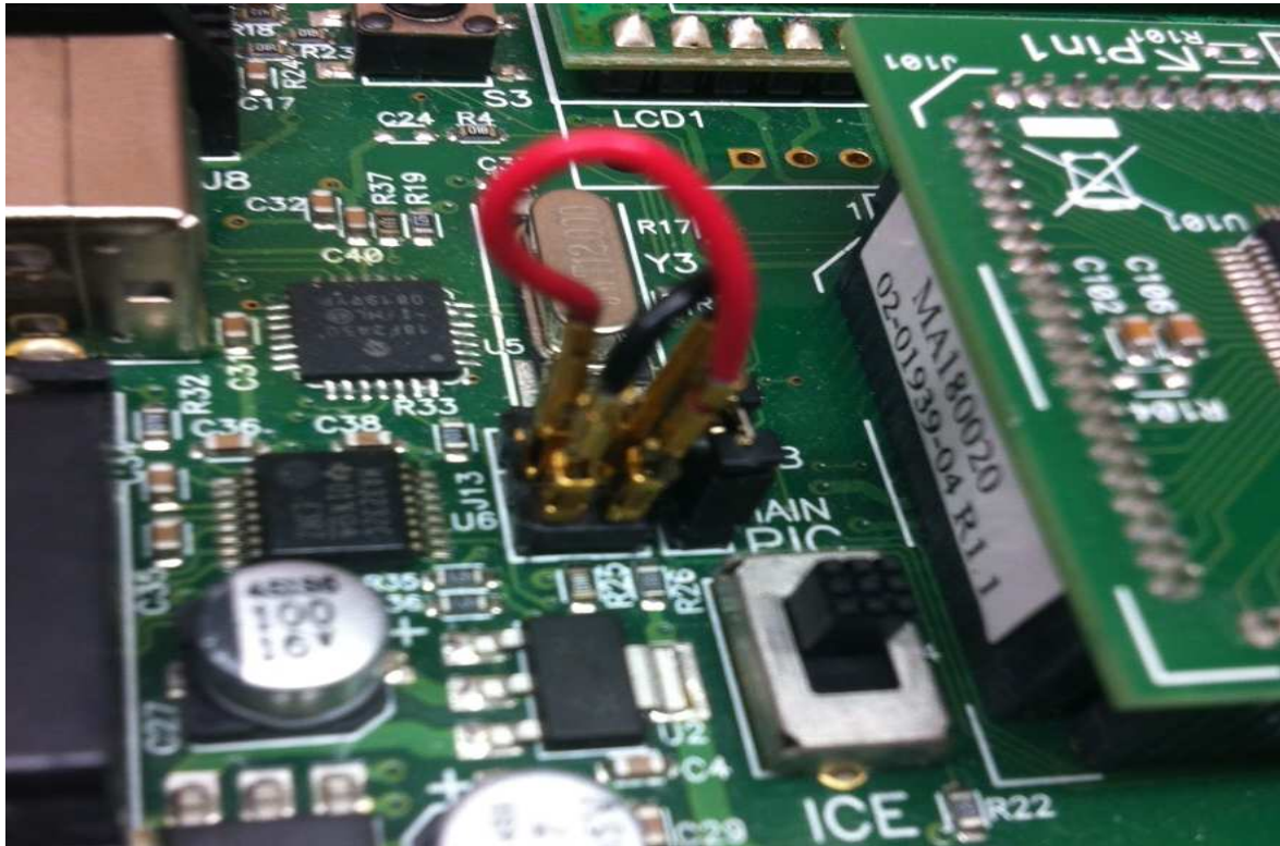
Figure 2. Jumper Selection for Command Mode Operation
