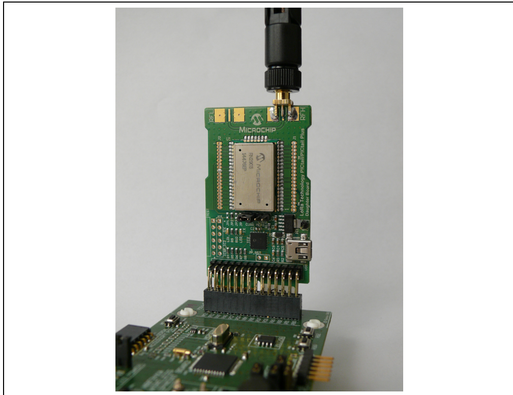
FIGURE 1-3: RN2903 LoRa™ TECHNOLOGY PICtail™/PICtail PLUS DAUGHTER BOARD CONNECTED TO PIC18 WIRELESS DEVELOPMENT BOARD
