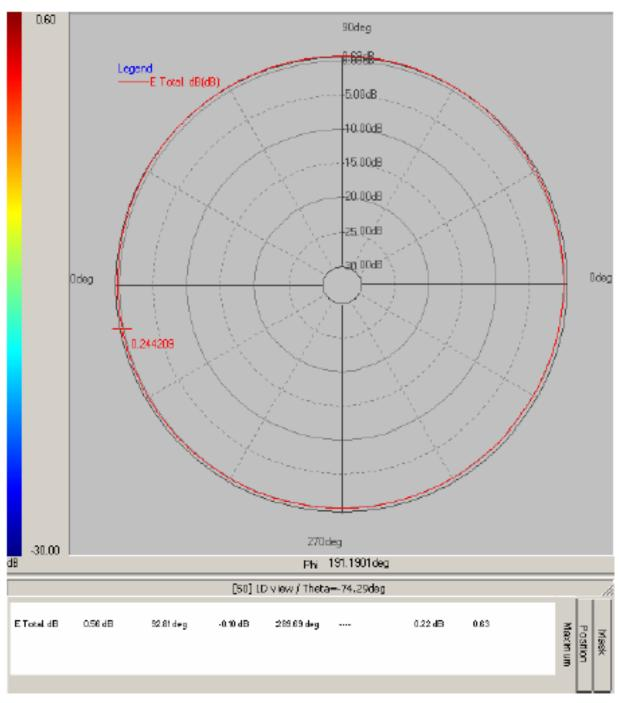
Frequency (MHz): 2450.00 Pattern Field: H Plane Average Gain: 0.22dB
