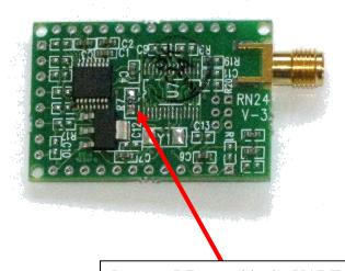
Remove R7 to enable the UART TTL signaling on pins 8-11. This disconnects pins 13-16 from the UART interface.
