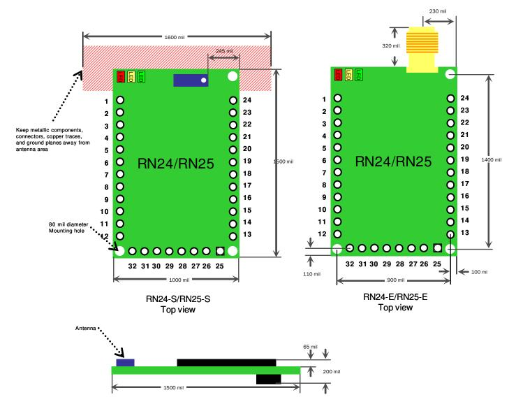
Connect with 24 pin DIP (through-hole) 0.1" pitch and 0.9" wide socket
