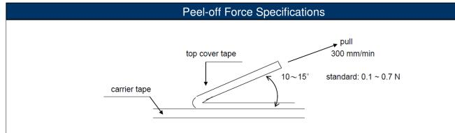
Peel-off force of paper and blister tape is in accordance with "JIS-C5202", that is, 0.1 to 0.7N at a peel-off speed of 300 mm/minute.
