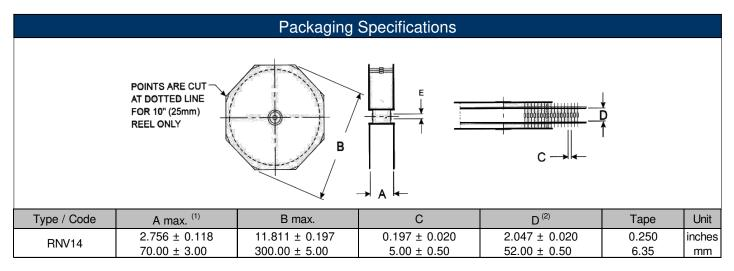
Dimension "E": This is a non-critical dimension that does not have a tolerance in the standard.
